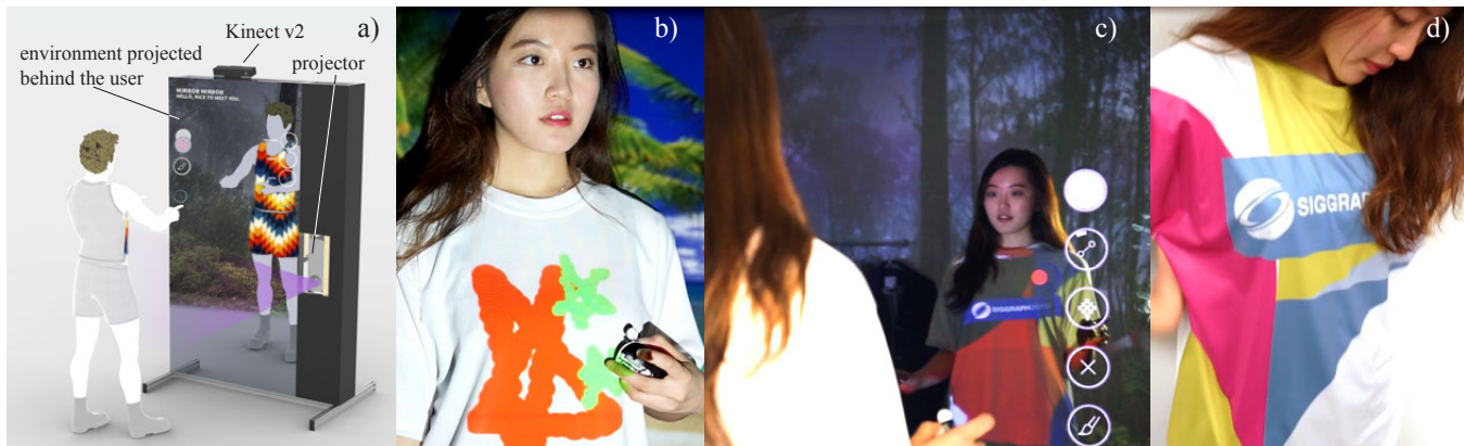
Figure 1: Mirror Mirror is a design system that combines spatial augmented reality with a mirror display (a). Virtual garments are visualized and designed both on the body (b) as well as in the mirror reflection (c) before being fabricated (d) with a fabric printer.
