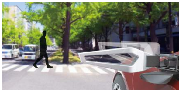
[Figure 1] We designed an actuated side-mirror to improve communication with other traffic participants.
