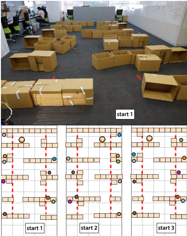
Figure 5: The search environment consist of a 5 \times 10 meter space filled with cardboard boxes. The red dotted line may not be crossed with the ground vehicle, in order to give the quadcopter enough room for turning. In this space, we laid out three configurations of equal difficulty. In the photo, configuration one is shown after a mission; some boxes moved due to collisions.
