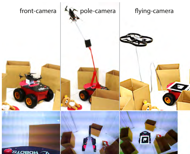
Figure 3: The three designs in the experiment. Shown on the left, a traditional front-mounted camera design in which an AR.Drone is mounted on top of the ground vehicle. The pole-mounted camera design is depicted in the center and has an AR.Drone mounted on an attached pole. Right, the flying-camera design. Here an AR.Drone is flying behind the ground vehicle. On top of the ground vehicle a fiducial marker is placed to estimate the position and orientation of the AR.Drone. The AR.Drone’s camera is used in all conditions to achieve identical video quality and intrinsic camera settings. The bottom row pictures show the respective views as seen through the AR.Drone’s camera.
