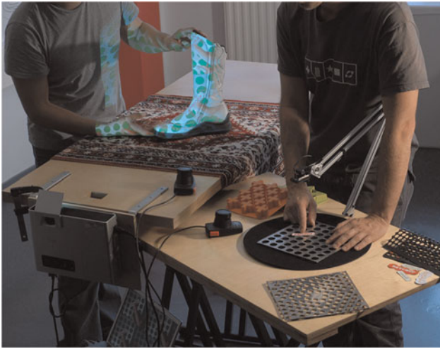
Fig. 3. The Skin setup consists of an object table, on which objects are illuminated with computer generated light, and a material palette for browsing and mixing visual materials. Physical materials are captured in real time with a video camera. Skin is designed to support small groups of designers in exploring and generating product concepts. [A color version of this figure can be viewed online at journals.cambridge.org/aie ]
