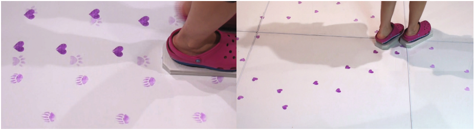
Fig. 1. The carpet is made from photochromic material that temporarily becomes dark purple under UV radiation. As shown, near UV LED embedded in shoes activate the color change long enough to create playful patterns.
