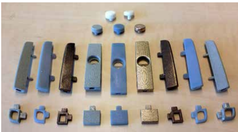
Fig. 3. 3D-printed components varying in shape (key holes and buttons) and material (gray: alumide, blue & white: plastic, brown & gold: steel).
