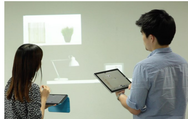
Figure 1: We studied how couples collaborate when designing in their living room. Our application consists of multiple synchronized tablets to manipulate objects, and a projector that projects the design real-time and real-scale on the wall.
