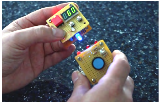
Figure 2. Modules connect in a network through outlets (blue LED) and inlets (red LEDs). Connections are made by holding an outlet near an inlet; the module cycles through the inlets to let users select a specific inlet. Through short range infrared communication, modules negotiate RF connection details. The LED is then lit solid, confirming an established connection. Disconnecting modules is achieved in a similar fashion, by again holding the modules together for a brief time.
