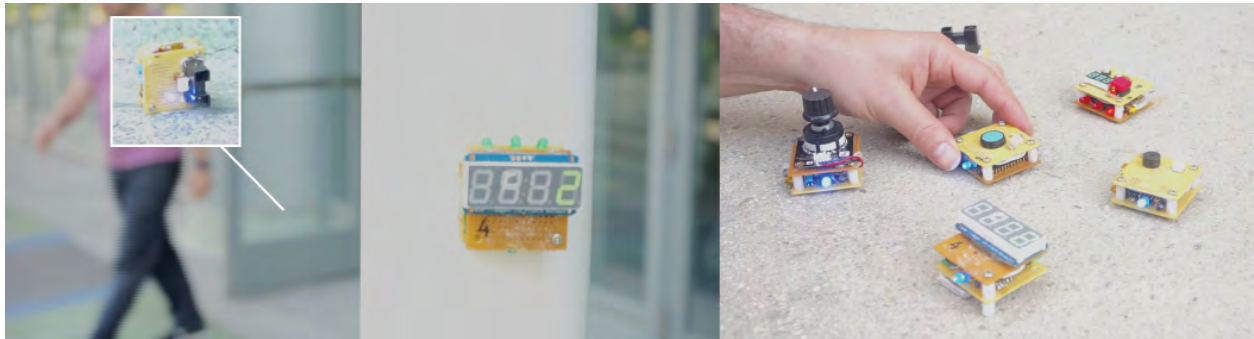
Figure 1. With Spatial Physical Computing (SPC) data processing modules are deployed in space and programmed with simple physical actions. Our prototype modules are battery powered and communicate wirelessly to form long range smart sensor/actuator networks. An example scenario is shown on the left: a proximity sensor generate events as a door opens, and a non-located accumulator module counts and display them.
